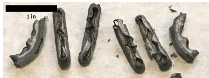
Figure 2.3. Six resistive heating samples of Al/PVDF/GNP at 15% solids loading GNP.
