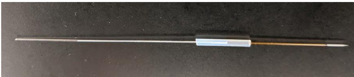
Figure 4.2. Photograph of capillary column (left) linked to a hollow needle emitter (right) using a PTFE sleeve
