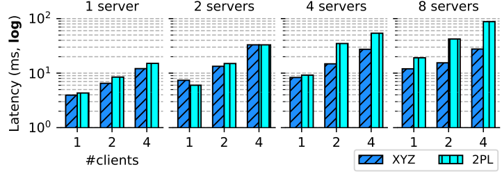
Figure 4.8.: Latency of an app using AEON’s protocol vs a two-phase locking in C++ with varying numbers of clients and servers.
