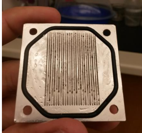
Figure A.1. Condensation surface for droplets in original prototype of selective condenser.
