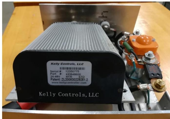
Figure 6.4. Inverter used in the testbench
