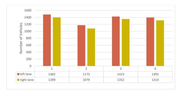
Figure 5.5 Comparing the number of vehicles on each lane at four different sections of the road at Patience 5 Seconds
