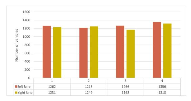
Figure 5.7 Comparing the number of vehicles on each lane at four different sections of the road at Patience 15 Seconds
