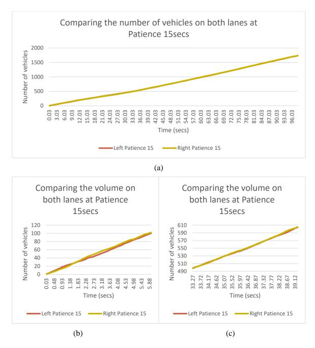
Figure 5.3 Comparing the Number of Vehicles on Both Lanes at Patience 15 Secs (a) showing the full simulation length, (b) - (e) showing the simulation in four sections
