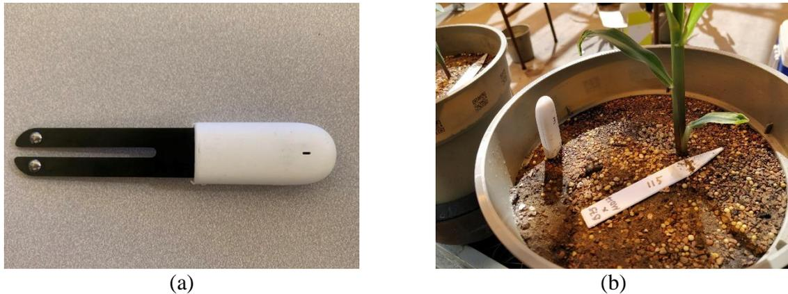
Fig. 2.6. (a). The layout of the Xiaomi Flower Care Sensor including temperature and radiation sensors; (b). The sensor was inserted into the soil of the pot during data collection.
