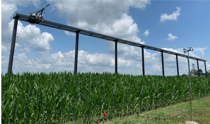
Fig. 5.1. Field VNIR hyperspectral platform at Purdue University. It consists of a VNIR hyperspectral imaging sensor (MSV-101-W, Middleton Spectral Vision, Middleton, WI, USA) and a local weather station (Ambient Weather, Chandler, AZ, USA). The gantry platform is seven meters high capable of scanning all or part of a 50-by-5 meter strip field under a wide range of weather conditions.
