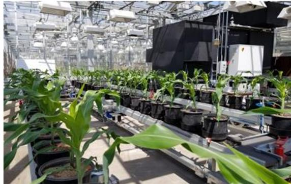
Fig. 2.2. Purdue Lily 13-4 Greenhouse with automated, high-throughput imaging system and a belt conveyor-based plant transportation system.
