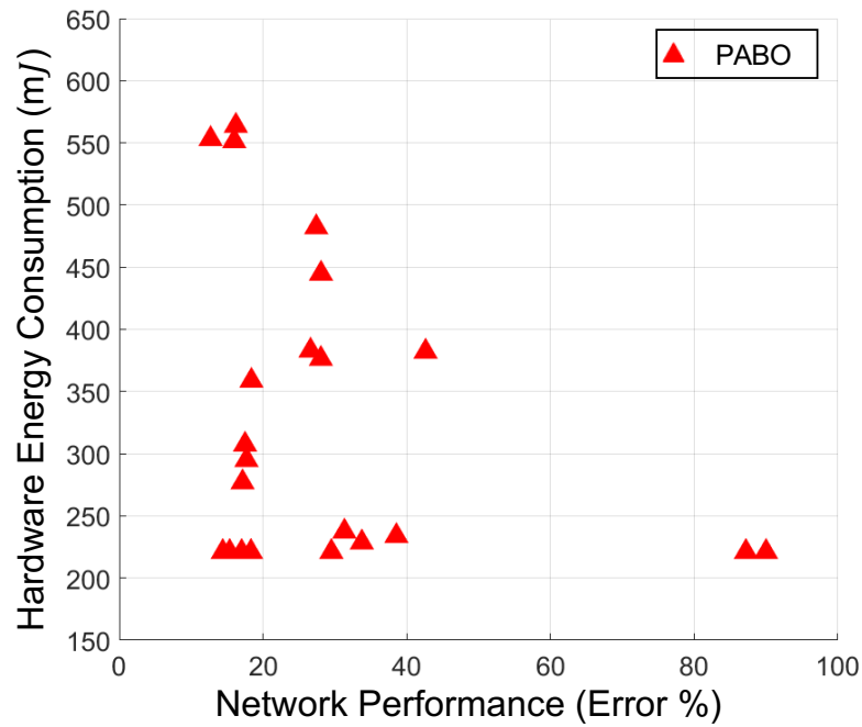
Fig. 4.6.: PABO for ANN on PUMA for case study three: VGG19 network on CIFAR-10 dataset with 3072 different set of HP combination. Other methods cannot be run on this case study due to significant computational requirements.
