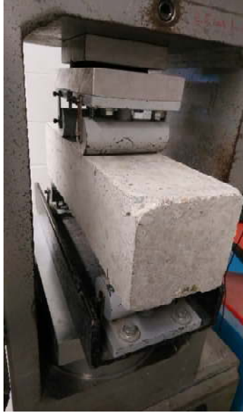
Figure 3-32 Test for modulus of rupture of concrete
