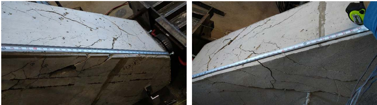
Figure 4-2 Anchorage failure of Specimen S-27-R11-L
