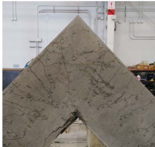
Figure 4-4 Crack maps and photos of Group S-2 specimens
