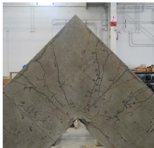
Figure 4-5 Crack maps and photos of Group S-3 specimens
