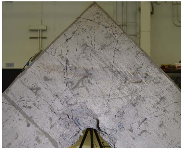
Figure 4-20 Crack maps and photos of C-Series specimens (Part 2)
