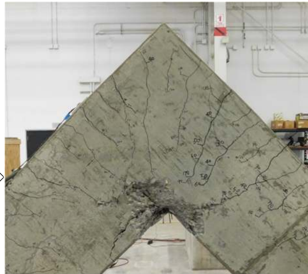
Figure 4-12 Crack maps and photos of Group D-1 specimens
