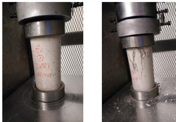
Figure 3-29 Concrete compressive strength test
