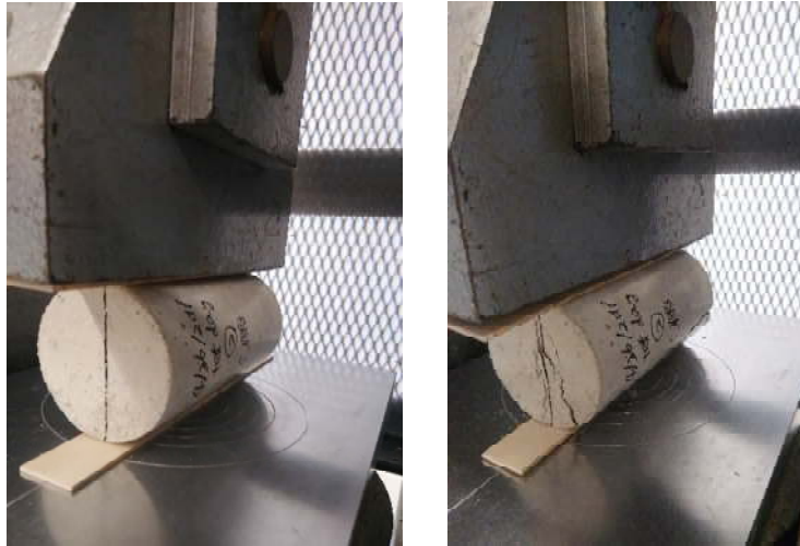
Figure 3-31 Test for splitting tensile strength of concrete
