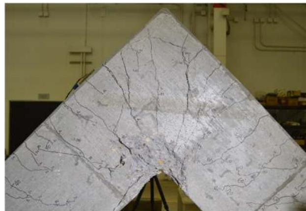
Figure 4-13 Crack maps and photos of Group D-2 specimens
