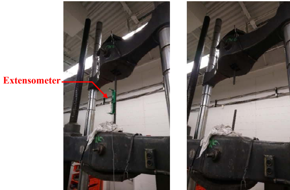
Figure 3-33 Test for tensile strength of reinforcement
