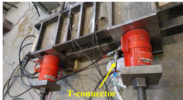
Figure 3-20 Hydraulic cylinders and T-connector with pressure transducer
