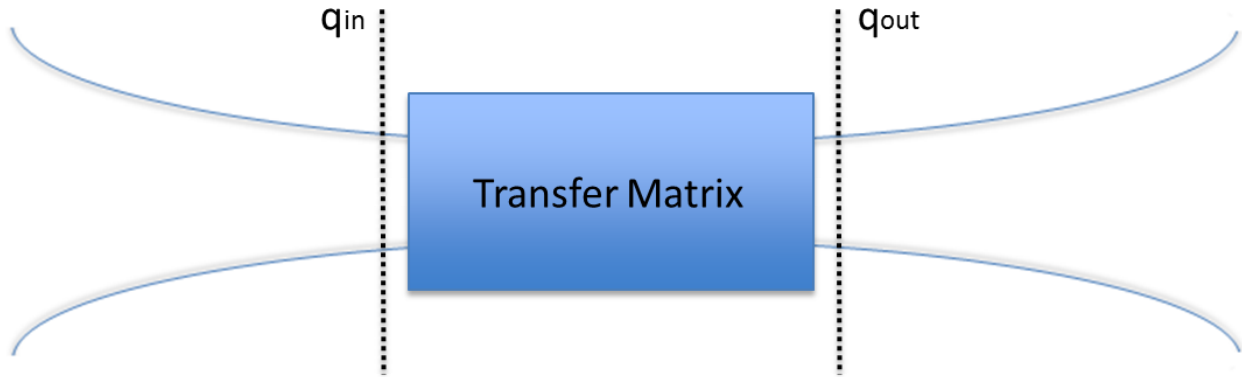
Figure 4.23. A representation of input and output complex beam parameters before and after a series of optical elements.
