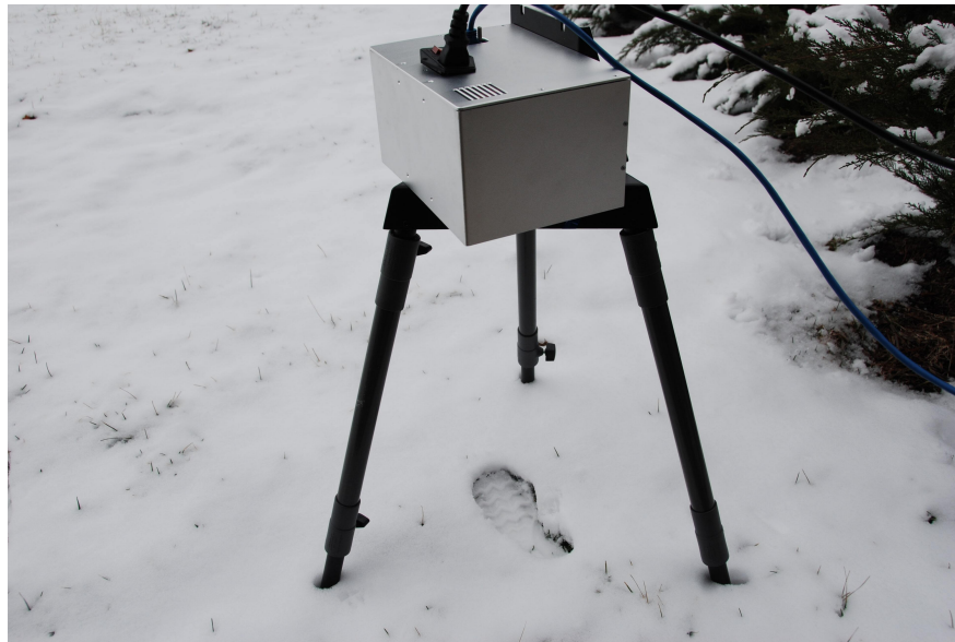
Figure 2.13. Prototype system set up above a shoe impression in the snow.
