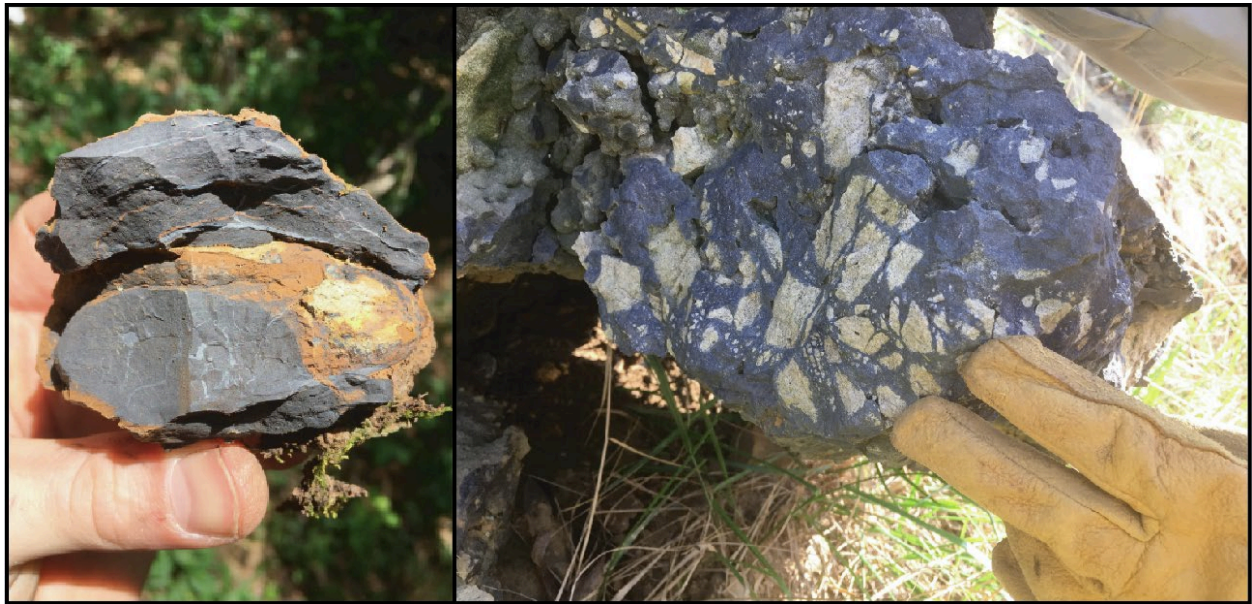
Figure 1.3. Field photos of common manganese oxide morphologies. Vein-filled botryoidal deposits (left) are common throughout Virginia. Manganese oxide-cemented breccias (right) are found both in Tennessee and Virginia, and frequently host dateable material. The botryoidal deposit was collected at the Silver Creek Mine, VA while the brecciated deposit was photographed at Gap Mountain, VA.
