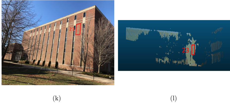
Fig. 4.18.: Planar features in the overlapping area between scans 5 and 6 displayed in images (a, c, e, g, i, k), which are captured by an external camera, and point clouds (b, d, f, h, j, l) (continued from the previous page)
