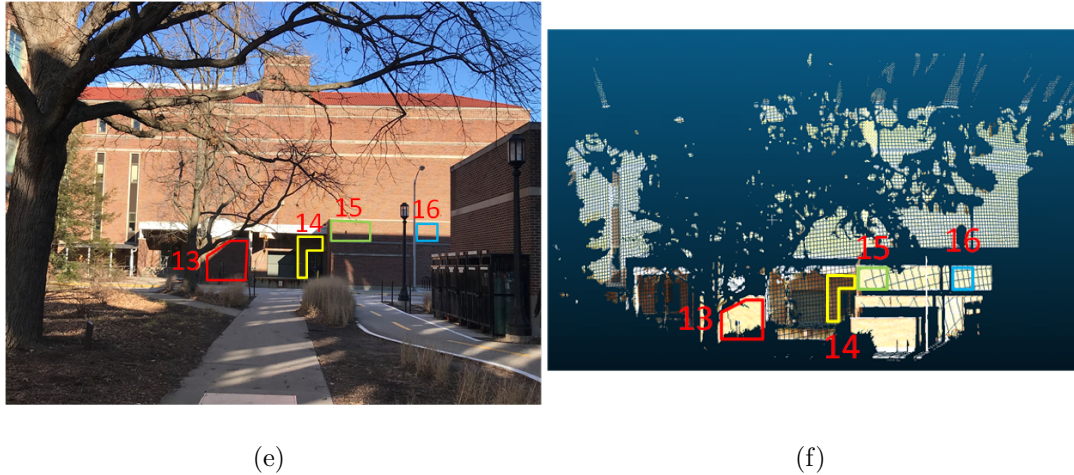
Fig. 4.24.: Planar features in the overlapping area between scans 7 and 8 displayed in images (a, c, e), which are captured by an external camera, and point clouds (b, d, f) (continued from the previous page)
