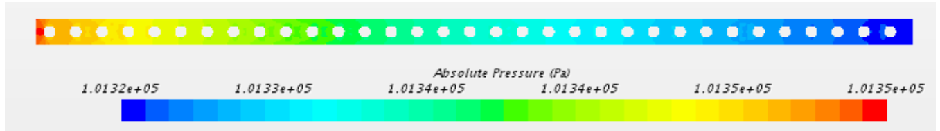
Figure S 4: Pressure drop results from CFD. L \times W \times H = 0.2 \text{ m} \times 0.006 \text{ m} \times 1 \text{ m} , N_{\text{coils}} = 33 , d_{\text{cooling coils}} = 3\text{mm} , v_{\text{in}} = 1\text{m/s} , T_{\text{in}} = 27^\circ\text{C} , RH_{\text{in}} = 70\% , T_{\text{coil}} = 10^\circ\text{C} , B = 5000 \text{ GPU} .
