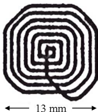
Figure 3.5: This real motion pattern was traced out on a notecard by the shaker with a marker attached. Settings were as follows: D1 = 1\text{ mm} , D2 = 13\text{ mm} , dD = 10 = 2\text{ mm} , Cruise speed = 16\text{ mm/s} , Acceleration = 200\text{ mm/s}^2 , and Current = 100%. This path differs from the ideal octagons dictated by the controller program because the stages take time to accelerate between rest and cruising speeds, a problem accentuated as the radius of motion becomes small, when octagons devolve into decreasingly rounded squares. In experiments, the shaker was set to describe large enough shapes to avoid momentary complete stops.
