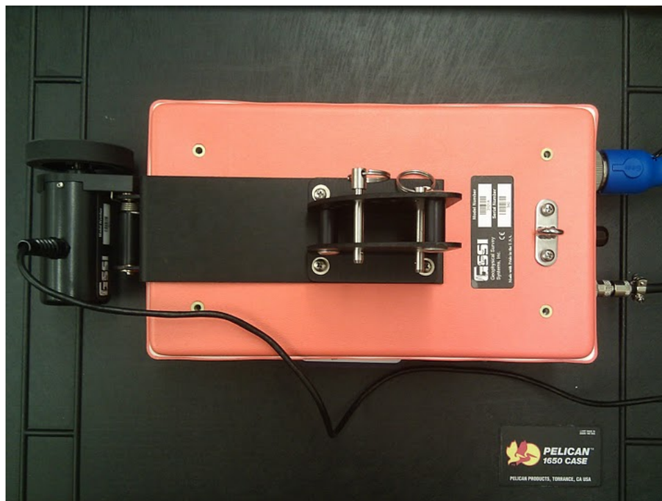
Figure 3.3.: Model 3101 900 MHz antenna attached to a Model 611 survey wheel
