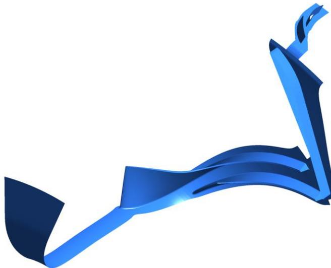
Figure 2.10 Computation domain used for numerical analysis of compressor stage
