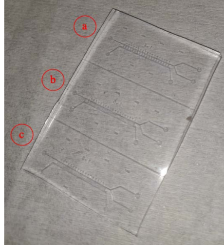
Figure 6. Prototype of PDMS layer containing 3 different microfluidic device designs. (a) Microfluidic design with rectangular protrusions magnetic structures. (b) Microfluidic design with rectangular bar magnetic structures. (c) Microfluidic design with rectangular bar magnetic structures with different spacing between magnetic bar and microchannel.
