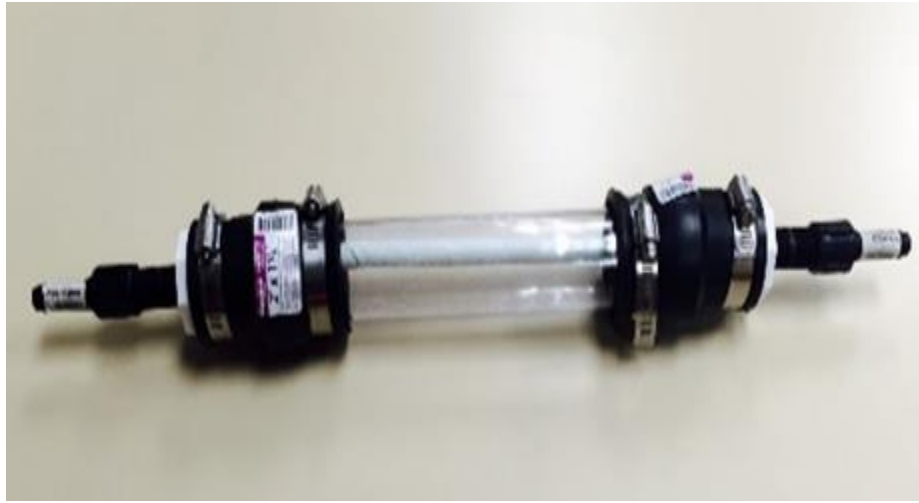
Figure 3.6. Assembled parts of the membrane module
