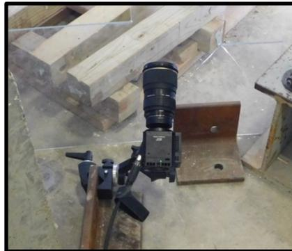
**Figure 3.27: High-Speed Camera**
