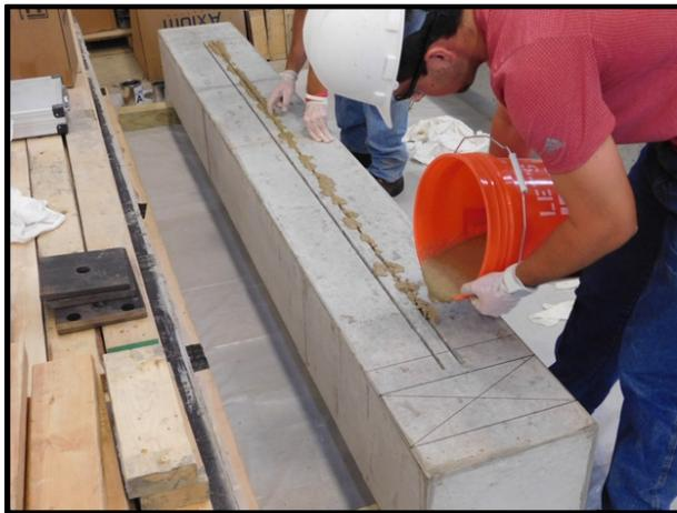
**(a) Filling Groove with Epoxy Grout**
