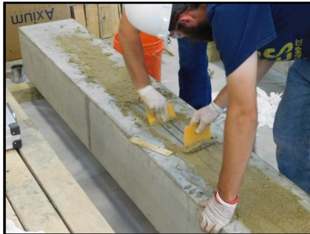
**(c) Squeegeeing Excess Epoxy Grout**
