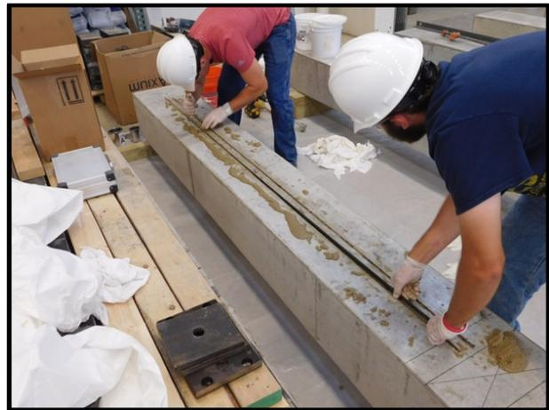
**(b) Inserting NSM Strip**
